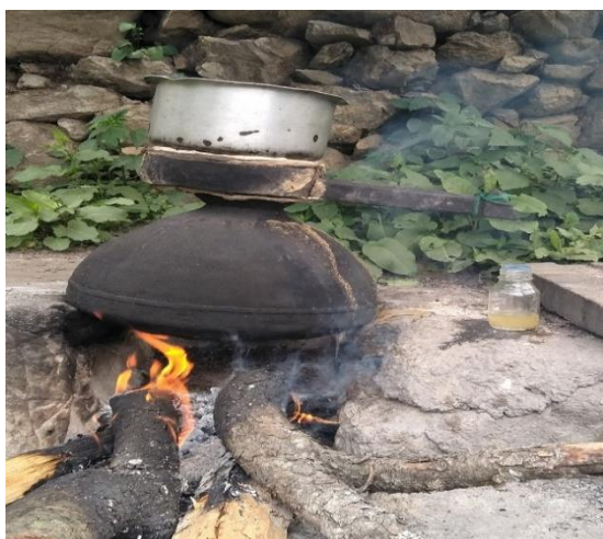
Fig. 3: Distillation assembly used in Jaunsar-Bawar region, Uttarakhand.
